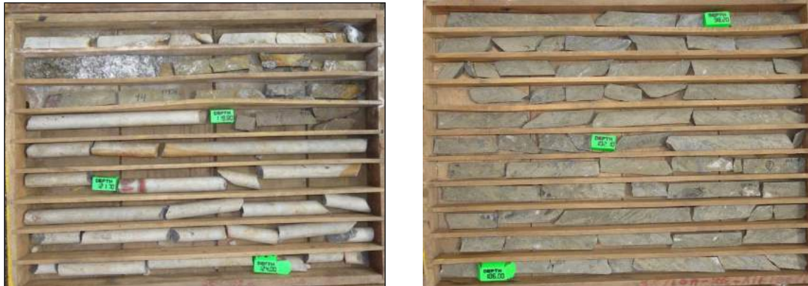
Figure 6.2 Examples of the State of Preservation of Gécamines Drill Core (a) base of the copper-rich Fault Zone and rare preservation of sterile dolomite in the footwall, and (b) massive zinc-rich mineralisation within the Big Zinc (drillhole 1270/9/V+30/-40/SE)
