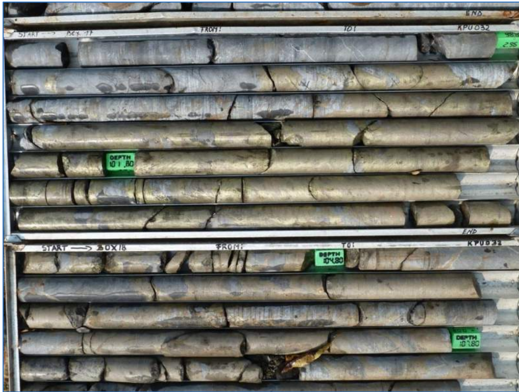
Figure 7.19 Drillhole KPU032 showing massive and patchy chalcopyrite/sphalerite mineralization in the Upper Kakontwe near the northern limit of the Fault Zone
