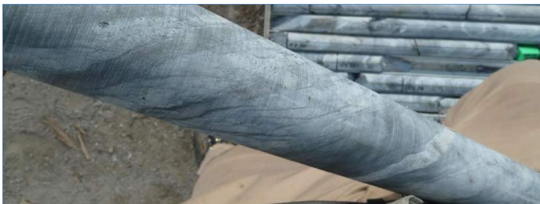
Figure 7.9 Interbedded Dolomite-shale/Siltstone Unit in the Upper Kakontwe Formation at 153 m in KPU070 (hole orientation -35 to 125). Bedding Dips Steeply to NNW (here in proximity to Kipushi Fault) and is cut by a Steep east-west Cleavage. Core is Positioned such that the Image Represents a Plan View with North to the top
