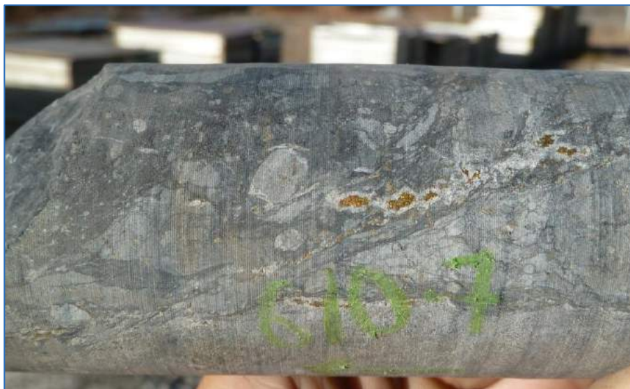
Figure 7.13 A carbonaceous/argillaceous-matrix breccia in the Upper Kakontwe <100 m east of the Kipushi Fault Zone. The clasts are dolomite and chert fragments with some brassy pyrite. The extent of structural fabric development varies considerably indicating deformation postdates breccia formation. 610 m in KPU002
