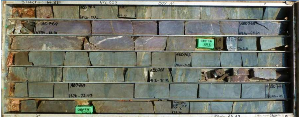
Figure 7.20 Typical colour variation in the Série Récurrente between dolomite (purple) and siltstone (green)
