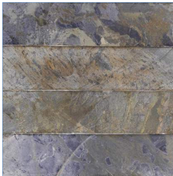
Figure 7.12 Sedimentary Breccia in the Kipushi Fault Zone from (top to bottom) KPU058 (77.4 m), KPU062 (82 m), KPU065 (87.8 m) and KPU066 (97.3 m). Pieces are 22 cm Long and Colour has been Enhanced
