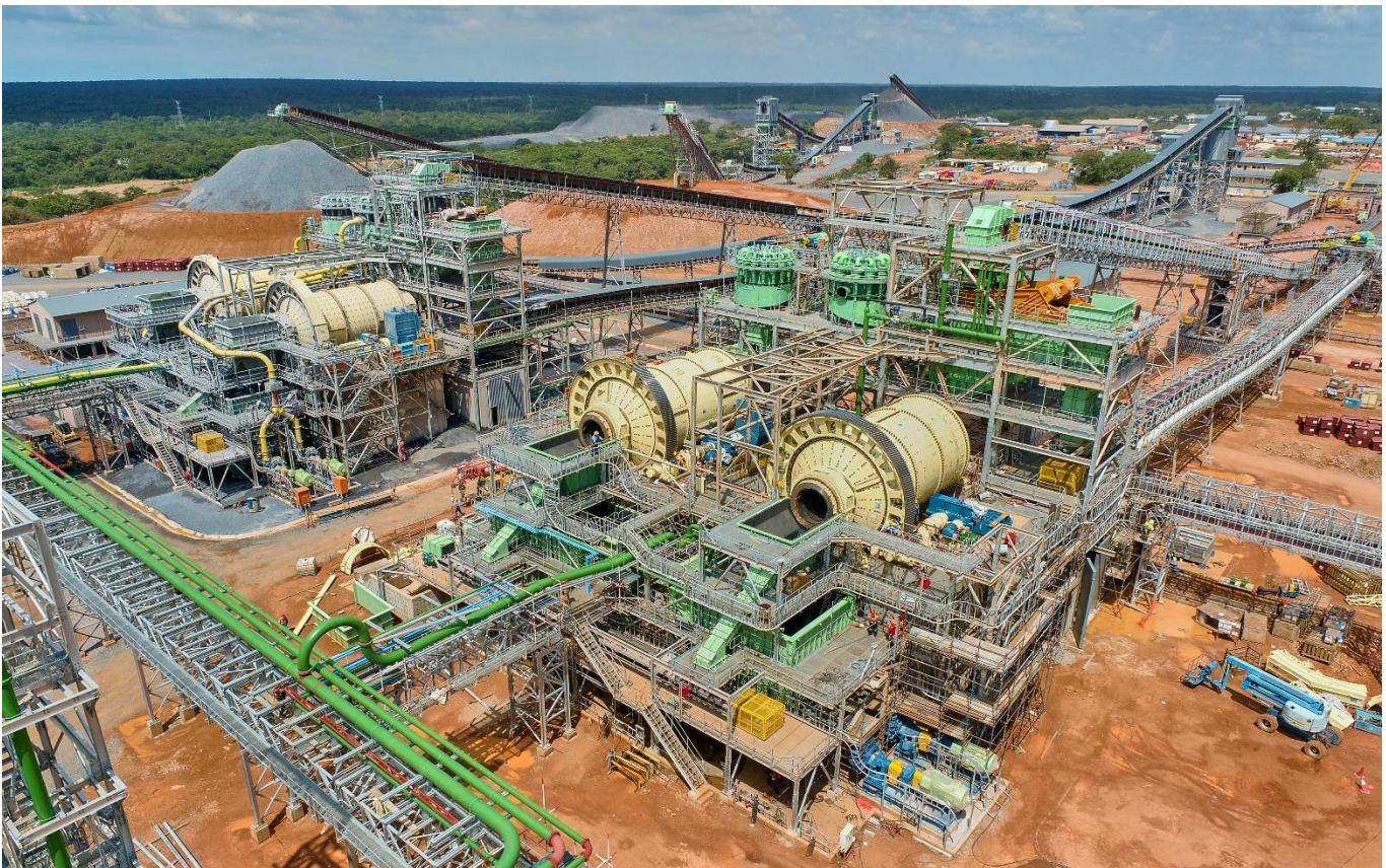
Kamoa-Kakula's Phase 1 (on the left) and Phase 2 ball mills.
