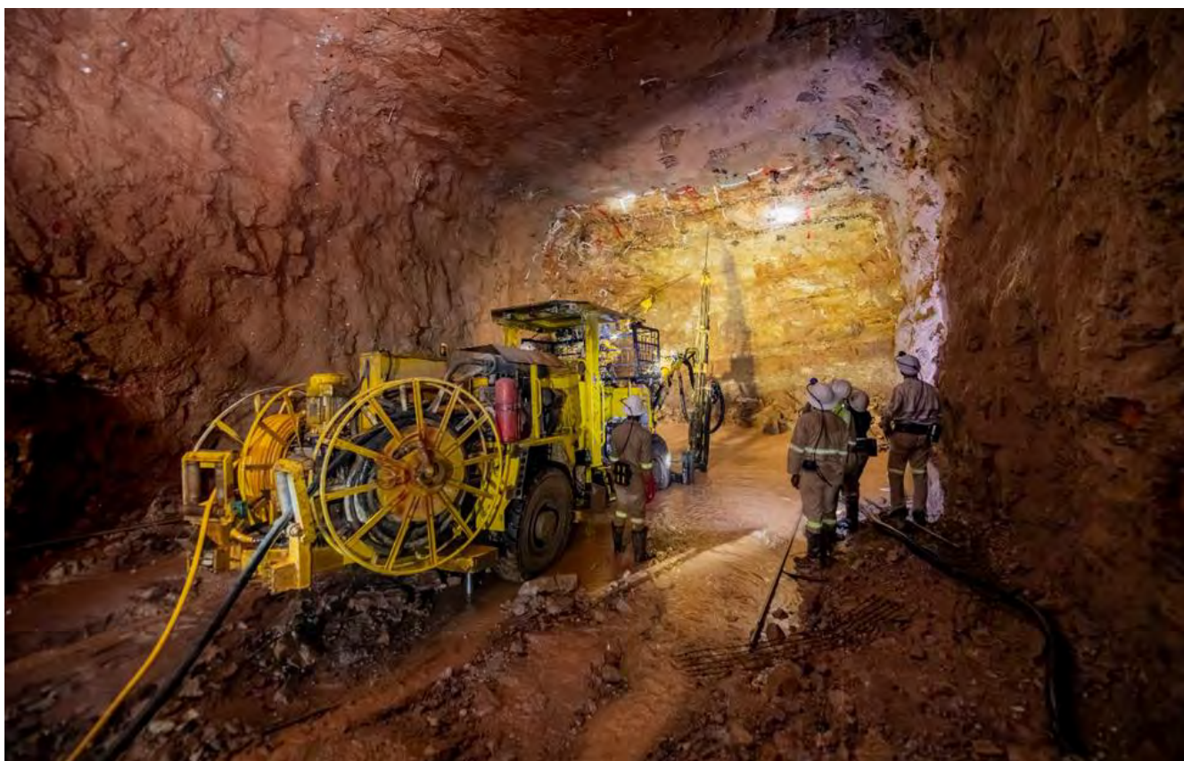
Photo: Kamoia 1 underground mining crew installing geotechnical support to the roof of an advancing development drive. The mining crews developing the new Kamoia 1 and 2 mines, as part of the Phase 3 expansion, recently achieved 365 lost-time-injury-free days.
